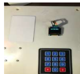
Fig. 7. Working prototype of Energy Monitoring System
