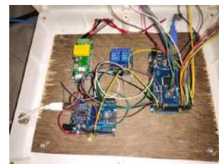
Fig. 6. Internal Connections of Energy Monitoring System Prototype
